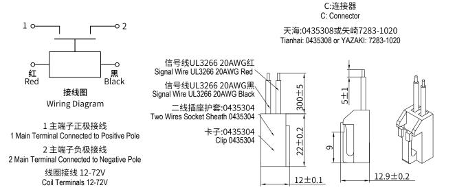
注: 产品主触头按接线柱旁标示 "1+" 的连接负载 "+" 端,接线柱旁标示 "2-" 的连接负载 "-" 端 Note: The product main contact "1+" which is marked near the bolt is connected to the load "+" terminal, and "2-" is connected to the load "-" terminal.
